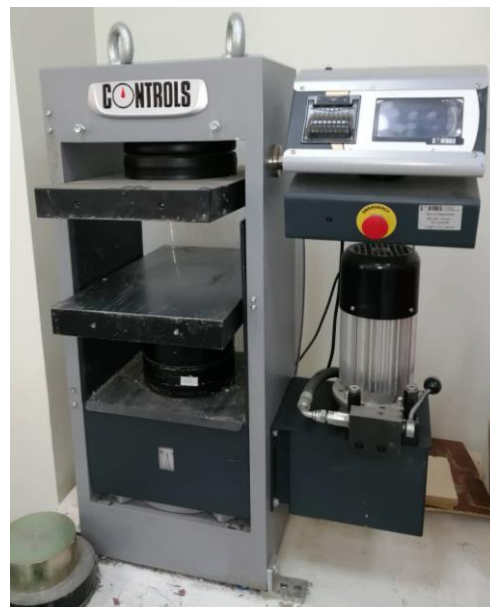
Fig. 3 Compression machine test
